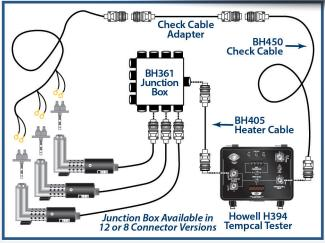
Harnesses containing up to 12 thermocouples can be tested by using the BH361 Series junction box. The H394 monitors the average probe temperature and the average thermocouple temperature.
