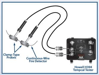
Clamp-type Probes (1 or 2 probes) are used to test continuous-wire fire detection systems such as those manufactured by Walter Kidde and Meggitt. These systems are checked by comparing the operation of the normal indicating device (indicator, lamp, alarm, etc.) with the heater probe temperature display on the H394.
