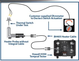
Thermal switches are tested by using a customer-supplied ohmmeter to detect switch actuation at the proper test temperature. BH405 heater cables are required for probes without integral cables.
