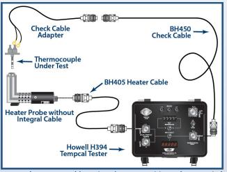
Thermocouples are tested by using the two position selector switch to compare the heater probe temperature with the output of the thermocouple under test.
